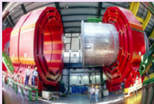
Initial assembly of the Compact Muon Solenoid detector. (Click on image for larger version.)
